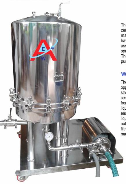
The AKSHAR manufacturer and supplier of zero hold up filter press in India that is made up of high quality stainless steel having customized finished design. The cartridge assembly consists of plates, perforated screens, spacers and fitter media stands on S.S. trolley. The whole assembly complete with attached pump and pipe lines through welding.
